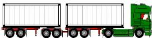
Truck TARW TPLC Semi Trailer + UV Headstock + TPLC Semi Trailer + Truck UV
